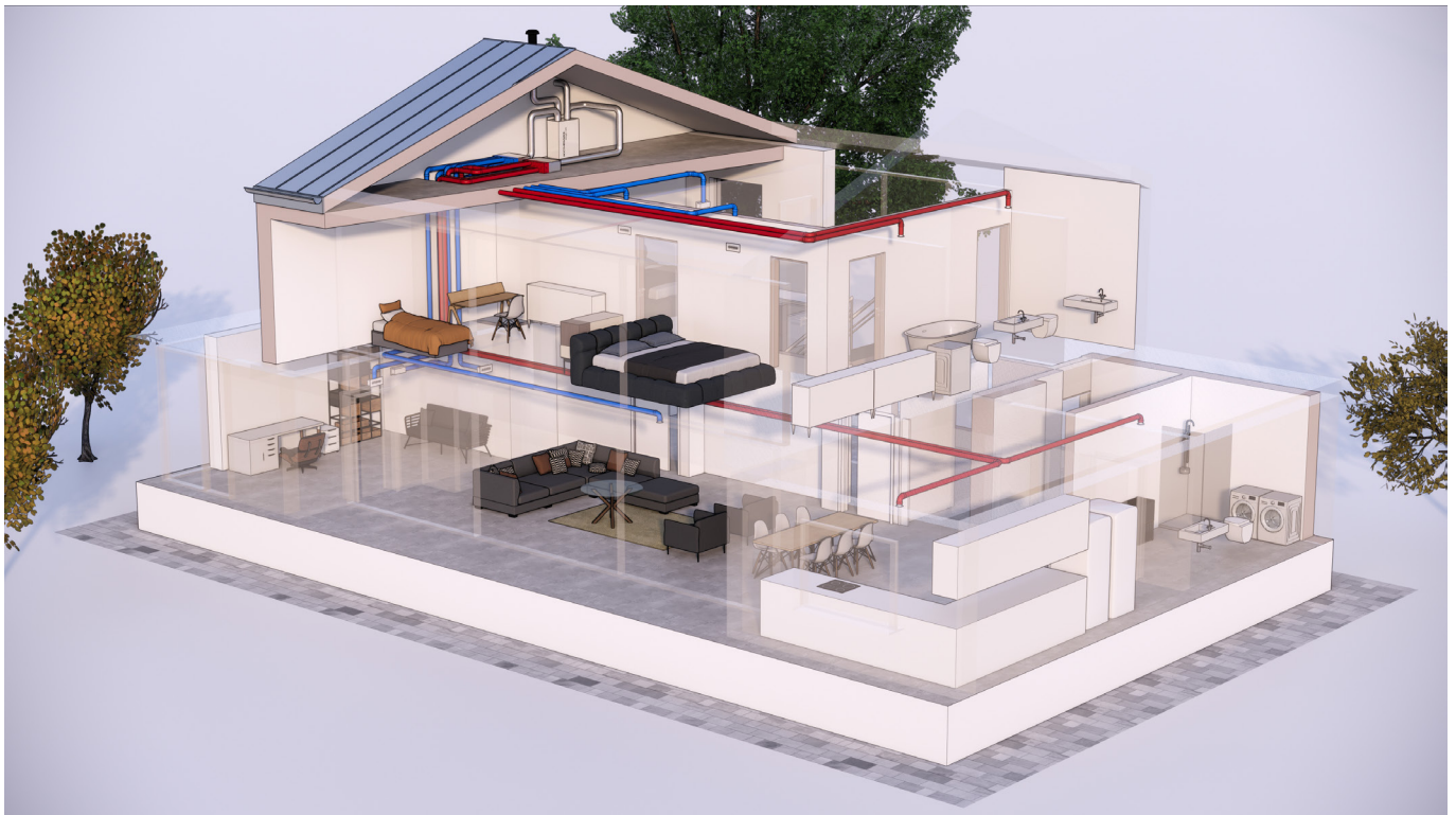
Example of DRU installation (vertical)
