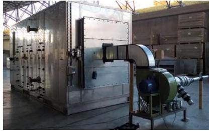
Leakage test according to EN 1886:2008
