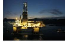
GVA 7500 (enhanced) Light NORSOK - ISO15138 Harsh Environment / Deepwater Semi-Submersible Drilling Unit Equipment delivered:
