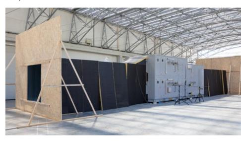
Noise test according to ISO 9614-1 Sound power level determination
