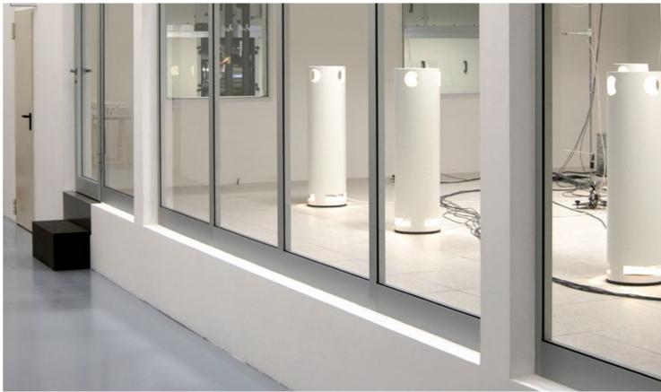
Among the first in the world to have a climate chamber, made according to the criteria of the EN15116 standard, the company has a test room for testing the performance of the air handling units.
