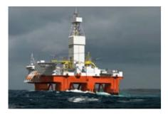
Moss CS60E Full NORSOK - ISO15138 Harsh Environment / Deepwater Semi-Submersible Drilling Unit
