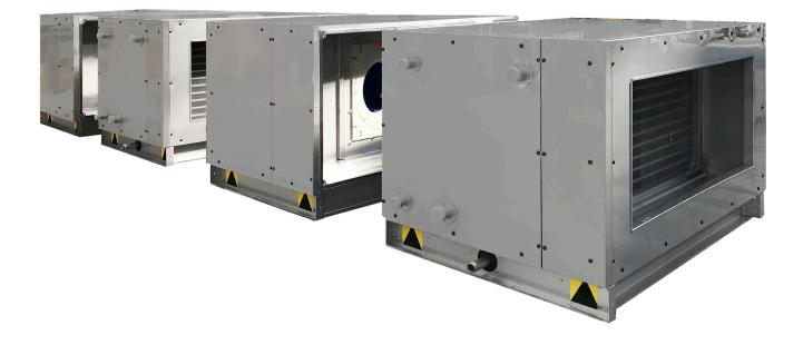
The sandwich-type panels with a thickness of 90 mm for the bottom of the sections and 54 mm for the side and top walls, are built on the inside in AISI 304 or AISI 316L stainless steel and, on the outside, in precoated galvanised sheet iron, with injected, high-density polyurethane foam insulation material (about 45 Kg/m<sup>3</sup>) or oriented-strand rock wool (about 90 kg/m<sup>3</sup>).
